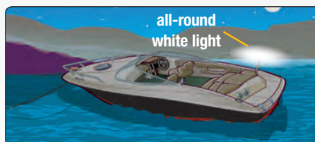
All-round white light indicating a vessel anchored away from the dock
